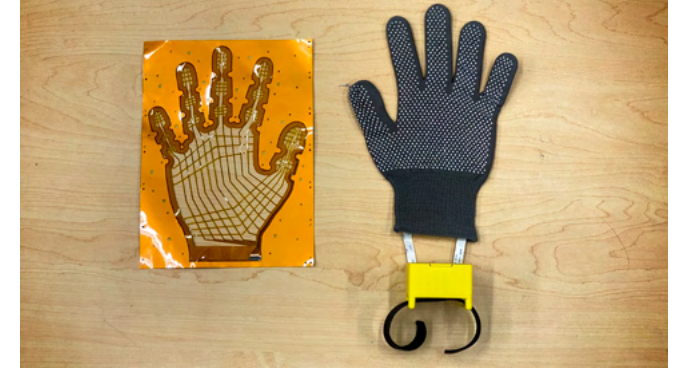
Inside the OpenTouch Glove (right) is a grid of wires (left) that allows the glove to sense the location and degree of any pressure applied to it. University of Washington
