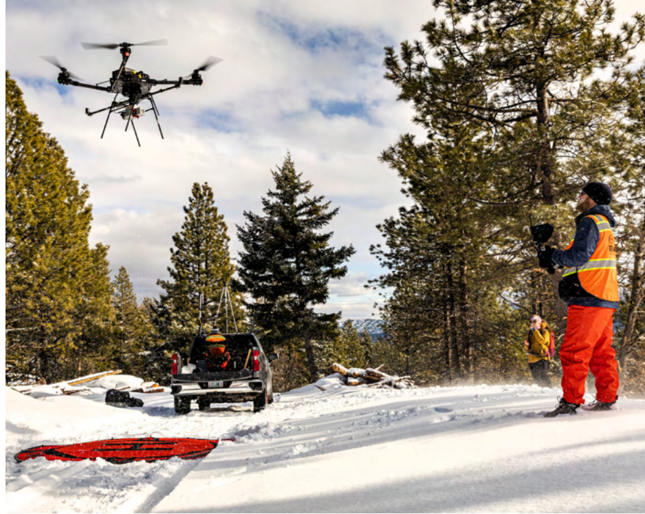
Researcher Andrew Lyda pilots a drone equipped with sensors to measure snow depth and forest density. Mark Stone / University of Washington
