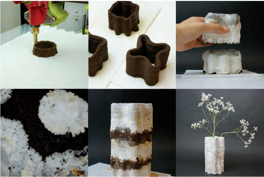
The stages of 3D printing a vase with a paste made of coffee grounds. Luo et al./3D Printing and Additive Manufacturing
