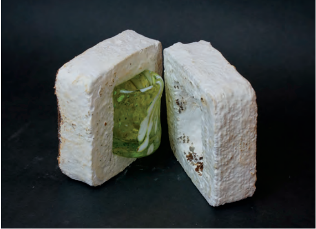
The compostable packing material around this small glass was 3D printed from used coffee grounds. Luo et al./3D Printing and Additive Manufacturing
