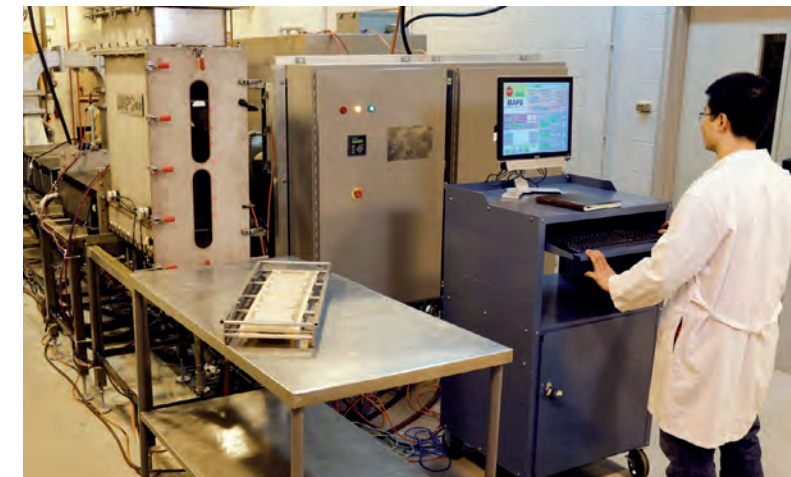
Engineers test an early prototype of the microwave-assisted pasteurization system that Juming Tang developed at Washington State University. Sabrina Zearott, WSU/CAHNRS Communications
