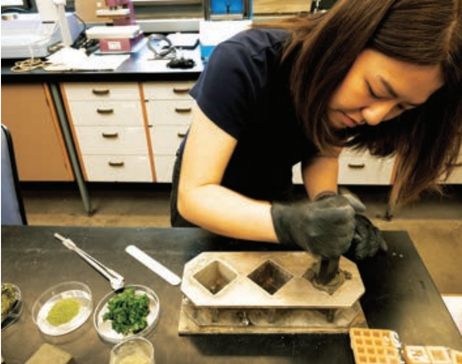
UW doctoral student Meng-Yen Lin casts green cement samples into molds to cure and later test their structural properties. Mark Stone / University of Washington
