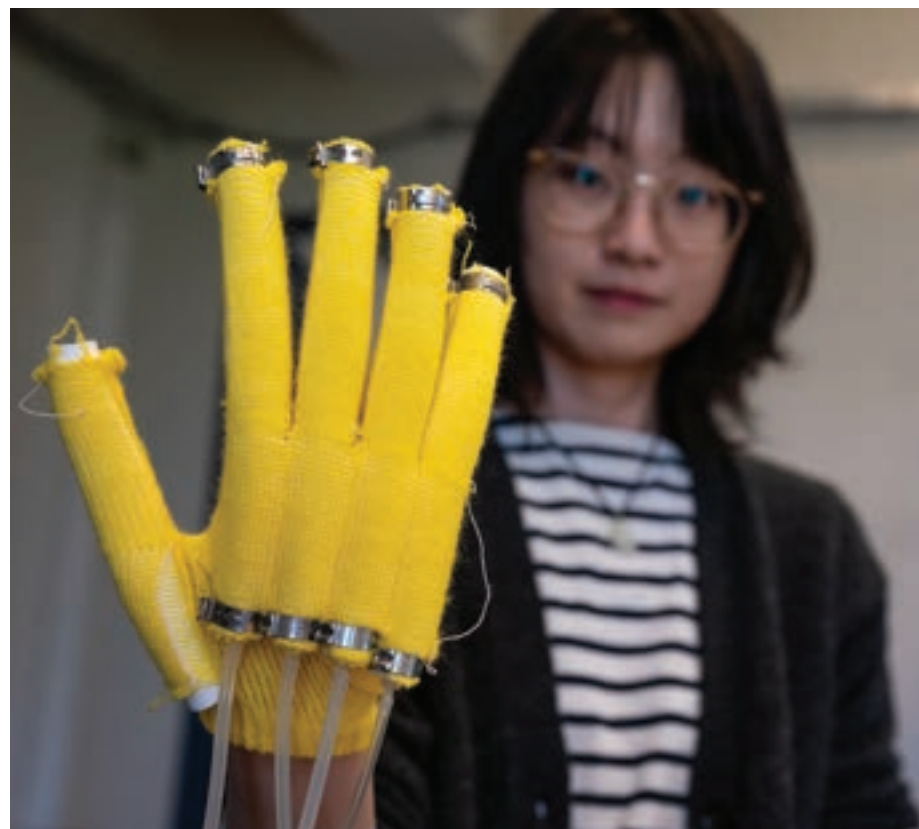
Yiyue Luo’s advanced tactile sensors, woven into wearables or worked onto robotic grippers, can accelerate imitation learning and policy training. Ryan Hoover
