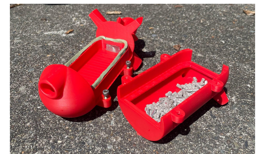
Figure 10: The submarine before testing, with the reaction chamber open and coated aluminum wire segments inside.
