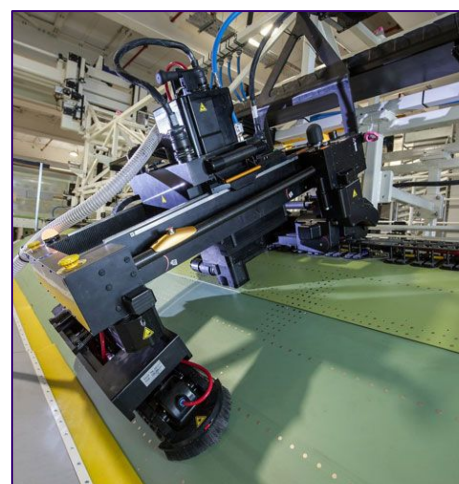
Flextrack 3.0 working on a curved component
