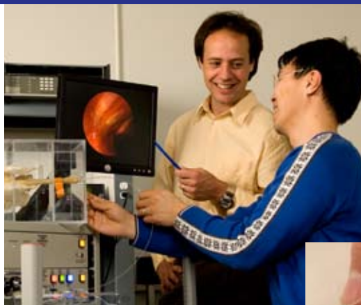
Above: Associate Professor Eric Seibel and ME doctoral student W. Jong Yoon examine an image of the broncheal lining of a dried pig lung, taken with the scanning fiber endoscope. Right: The capsule holding the scanning device is only 16-mm long.
