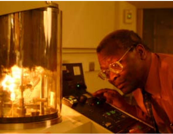
Sam Jenekhe , Boeing-Martin Professor of Engineering and professor of chemistry, is using nanotechnology methods to develop organic solar cells with self-assembled polymer nanowires. He watches a thermal evaporator complete the final steps of fabrication.
