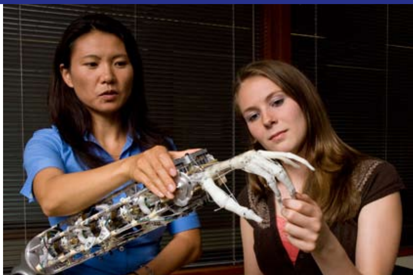
Associate Professor Yoky Matsuoka and undergraduate Carissa Conway examine the robot hand, a step toward a lifelike prosthesis.
