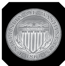
High-resolution image of the UW seal created by electron beam lithography. Several hundred would fit on the end of a human hair.
