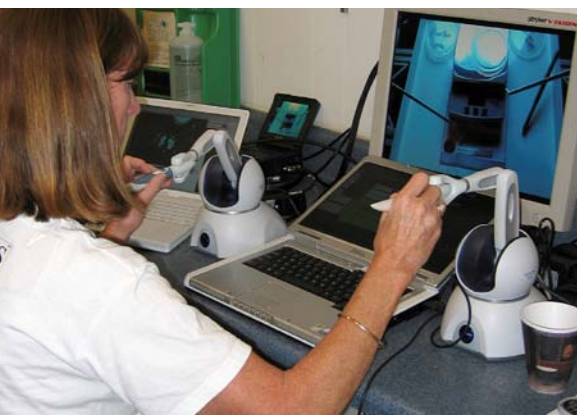
During the NEEMO mission, Raven did double-duty as a lunar sample manipulator. Mary Sue Bell, a planetary geologist at the Johnson Space Center, controlled the robotic arms to test Raven's ability to manipulate simulated lunar rock samples (right foreground).
