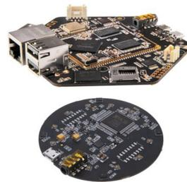
A microphone array is used to collect audio, the array allows for spatial information to be collected. The direction of arrival of the signals assist in noise reduction and speaker identification. Beamforming takes the direction of arrival so that sounds from different directions can be suppressed (noise) or enhanced (speakers).
