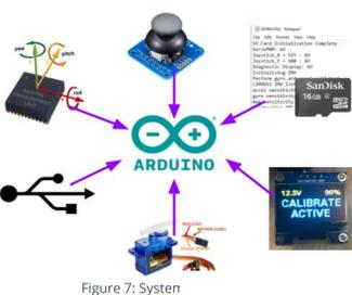
In Figure 7, above, all components of the design were integrated through Arduino. These include SD diagnostics, internal display, servo PWM, IMU sensor fusion, serial USB diagnostics, and pilot joystick passthrough.
