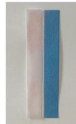
(left strip) that is exposed to water, whereas (right strip) is not exposed to any sources of water.
