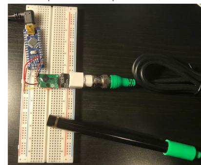
Conductivity sensor operating separately with Arduino Nano in UART mode
