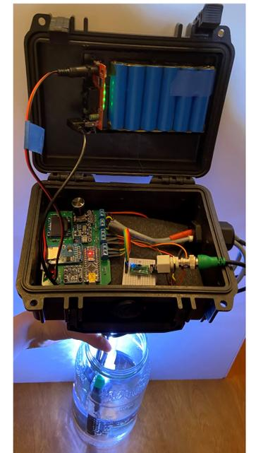
Integrated Smart Light Trap with conductivity sensor
