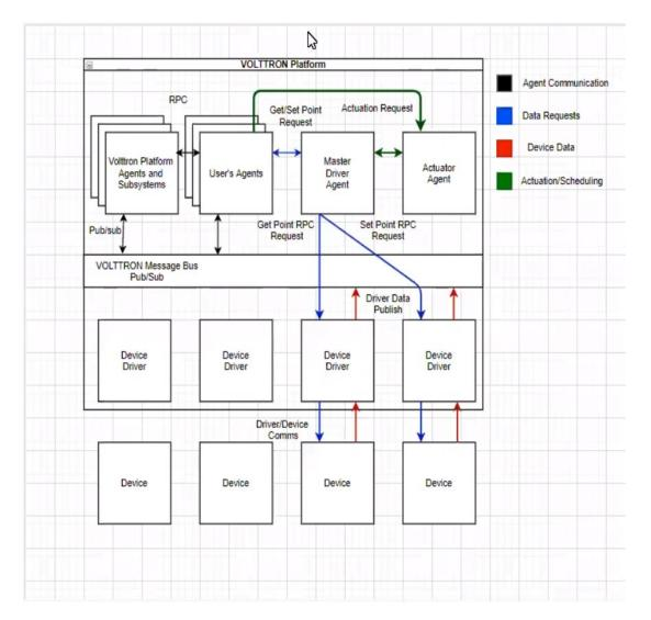
Bacnet specify one to many relation network requriemnt, Proxy Agent was used to handle communications. In our case, we have AHU only (air handler unit as our device).
