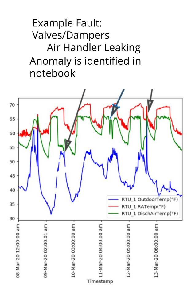
• Analytics so far rely on physics based models or logic checks to determine
