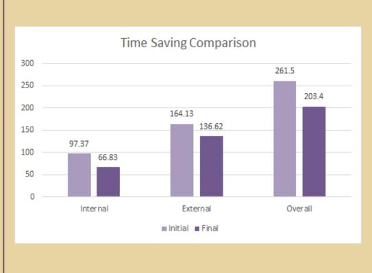
Final time study data with new fixture only had 6 samples however, it gives a rough estimate of the time saved. Based on the data collected, the is an estimated 22% time savings however, we predict around 15% time savings based on variability of tubes and limitations of the time study samples.
