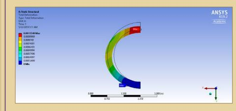
• Test case: Largest tube OD, smallest wall thickness, weakest material
