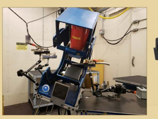
Quick clamps fixture with two grooves provides more freedom for orienting tubes for X-ray imaging. Inefficient movements for setup could be avoided.
