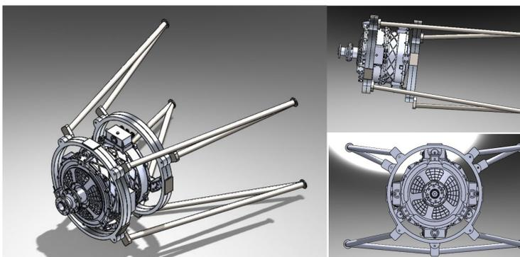
Final CAD model of Magni-500 engine mount, showing isometric (left), right (upper right) and front (bottom right) views
