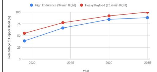
Change in flight time with constant hopper capacity (including 30 min reserve)
