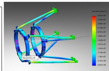
Von Mises stress plot of nominal torque simulation
