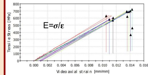
Total of eight dog-bone specimens trimmed from top and bottom panels were tested with "Instron 5585H 250 kN electromechanical test frame" to find the physical properties of the thermoplastic composite, utilizing measurements of axial stress and strain.
