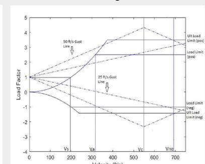
The graph above shows the flight envelope of the Boeing freighter aircraft. Once pushed outside of the bounds of these lines, the aircraft will either stall or sustain structural damage.
