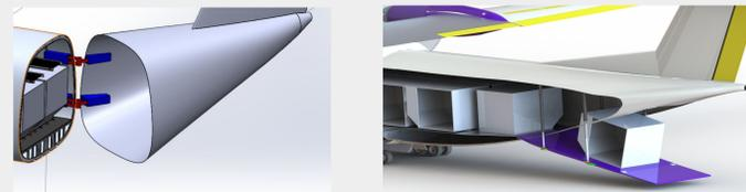
Swing-tail design produces issues with maintaining electrical, hydraulic, and fuel connections
