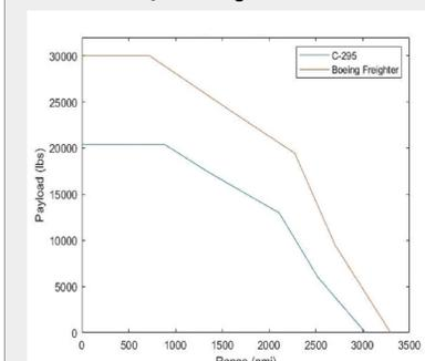
This chart shows the range and payload trade-offs that are feasible for our Boeing aircraft. It is compared to a C-295 which is a military turboprop cargo aircraft similar to our design.
