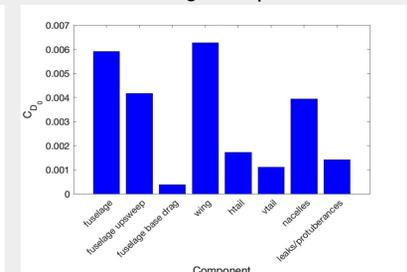
A breakdown of the parasitic drag contribution for each major aerodynamic component of the aircraft is shown above. The zero-lift drag does not include drag generated by 3-D effects.
