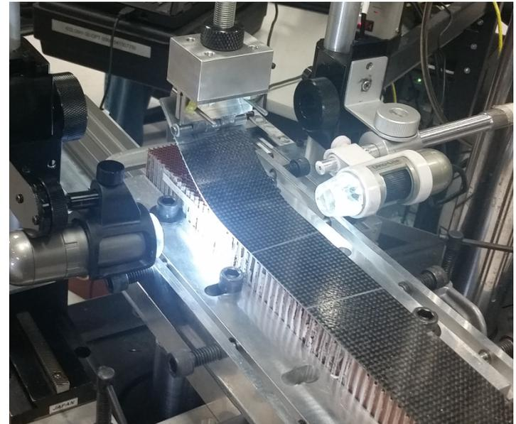
Single Cantilever Beam (SCB) sandwich specimen used to measure Mode I Fracture Toughness
