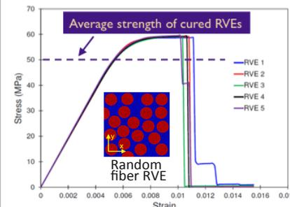
Response of fiber-matrix RVE under transverse tension - with and without effect of processing
