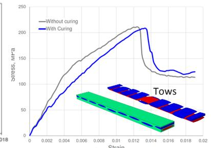
Response of 8-harness satin weave strip under transverse tension - with and without effect of processing
