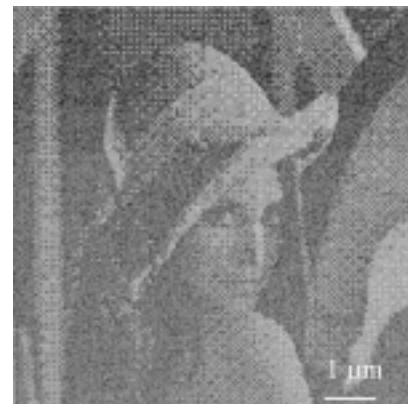
Fig.2 Ferroelectric data storage with the density of 717 Gbit/inch 2 in CLT. This figure is composed of 256X256 nano-domain dots with a bit spacing of 30 nm.
